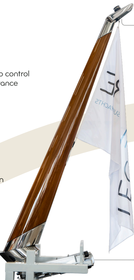
Automatic or manual rotation system that's lockable
